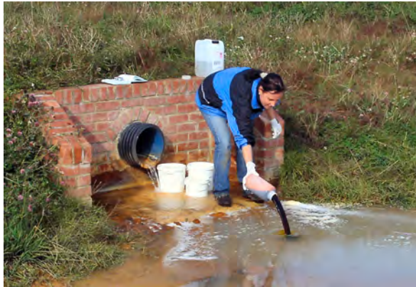
Figure 5: Injection of the Na-fluorescein tracer into RAPS II.
