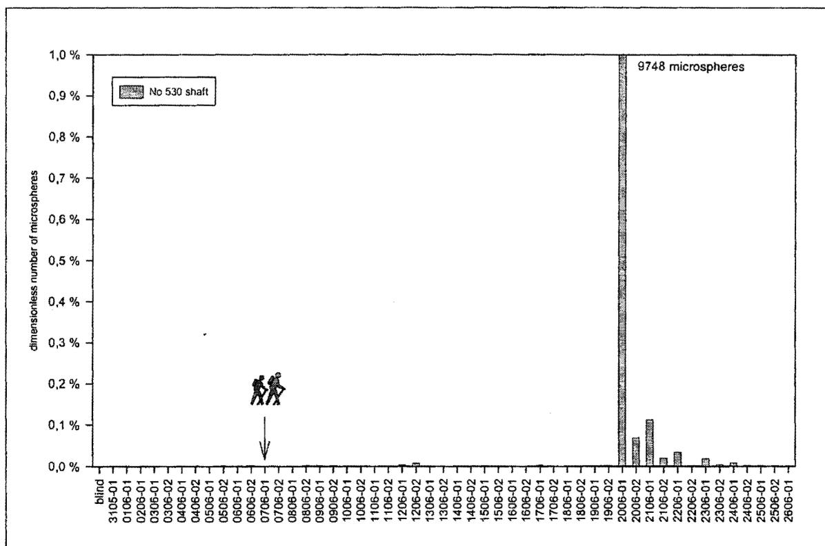
Fig. 5: Breakthrough diagram of the microspheres detected at the Glasebach shaft (max.: 9,748 microspheres). Arrow marks time of tracer injection.
