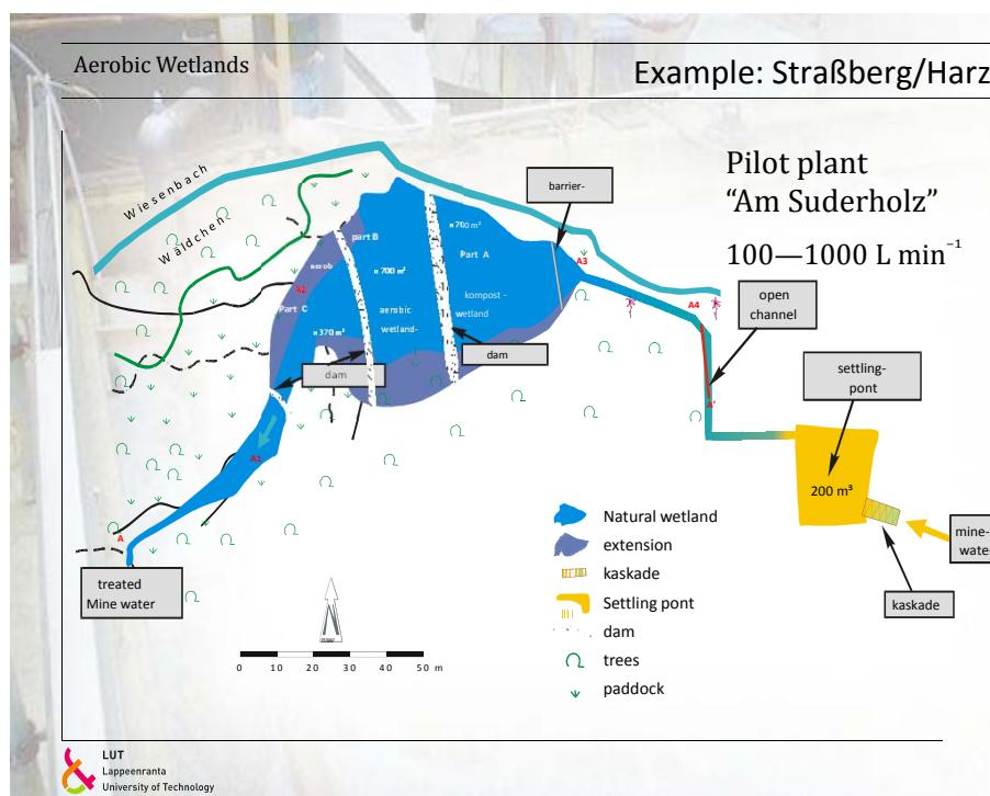
Passive Treatment      Aerobic Wetlands: Plants' Iron Removal (1/4)
