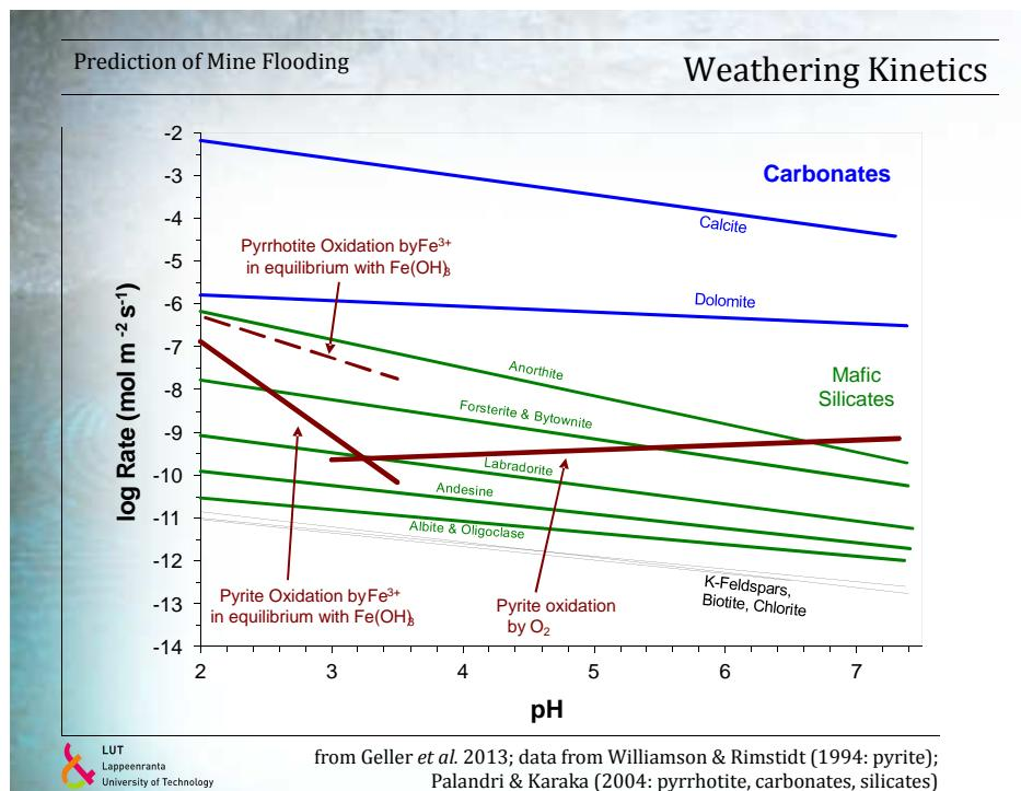
Prediction of Mine Flooding      Weathering Kinetics
