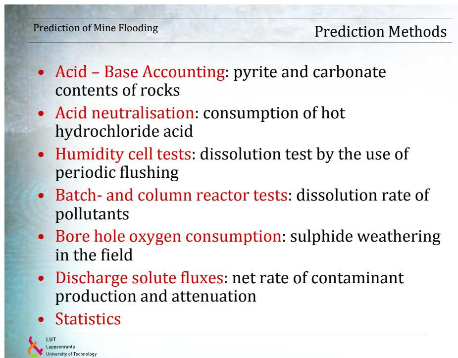
Prediction of Mine Flooding Acid-Base Calculations
