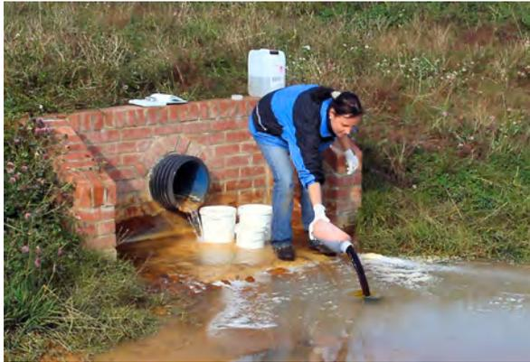
**Figure 5: Injection of the Na-fluorescein tracer into RAPS II.**
